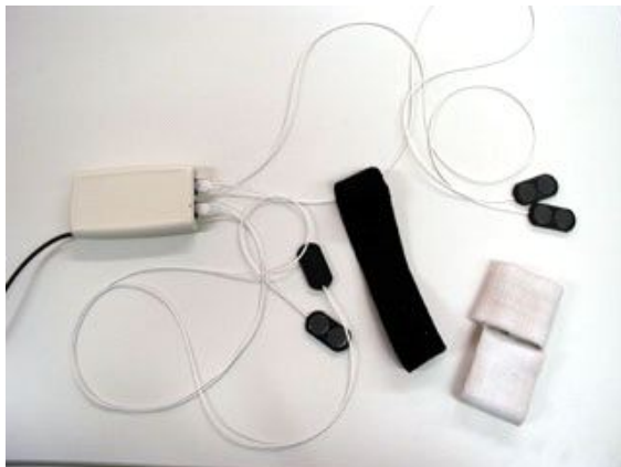
Figure 2: Complete Standard equipment: Main unit, Electrodes, Head band and Wristbands
